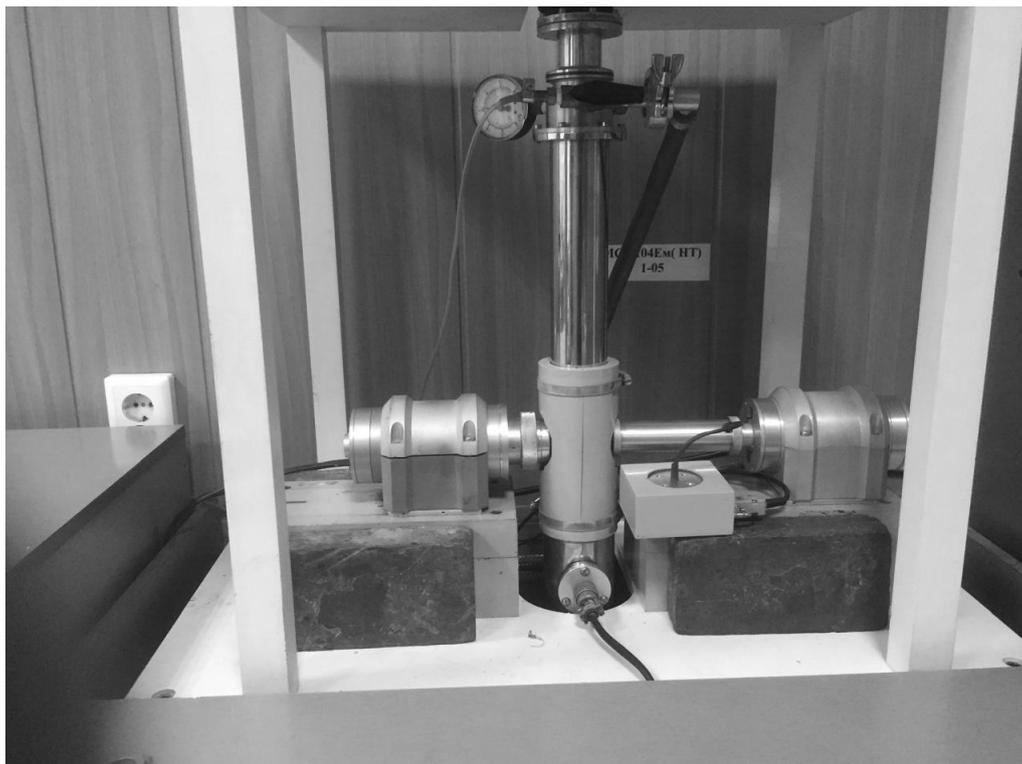
*Fig. 2. Mössbauer spectrometer MS-2020 with double modulation and helium refrigerator*
