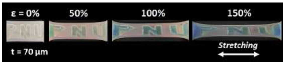
Fig. 1. Photographic images of CLCE film showing “PNU” letters as it is stretched.
