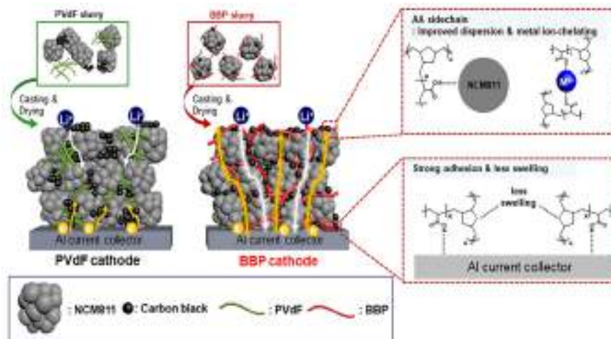
Fig. Schematic of the amphiphilic bottlebrush polymeric (BBP) binders for scalable high-areal-capacity Li battery cathodes.
