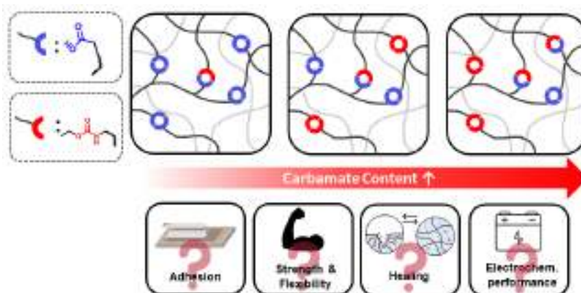
Fig. 1. Schematic representation of the various H-bonding interactions in the binder in proportion to the carbamate content and the properties that are influenced by the carbamate content.
