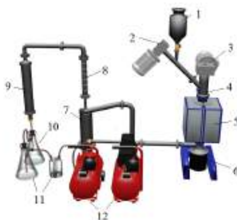
Fig.1. Experimental setup for the flax shive fast pyrolysis process
