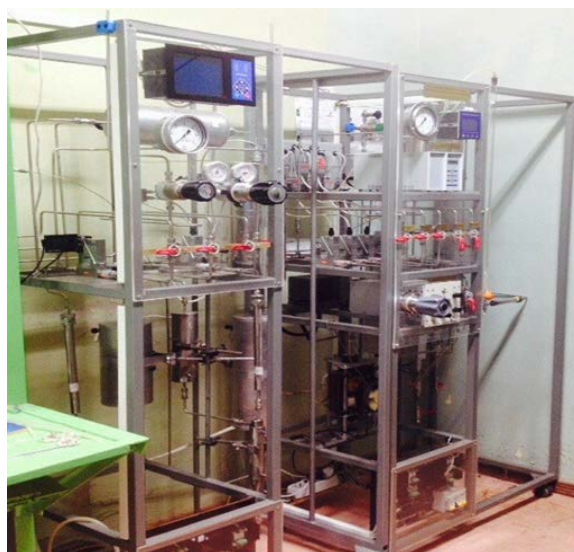
Pic. 1 – The monocyte, test complex of conversion of natural and associated petroleum gases (APG) into synthetic hydrocarbons by the Fischer - Tropsch method
