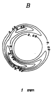
Fig.1 The spatial distribution of radical I in cylinder granule of catalyst support (type I) as a result of mass transfer process from the solution of radical in CCl_4 into the granule preliminary soaked in pure solvent. The starting conditions are in accord with nonequal distribution of solution around the granule. The spatial distribution presented as a relief surface with amplitude
