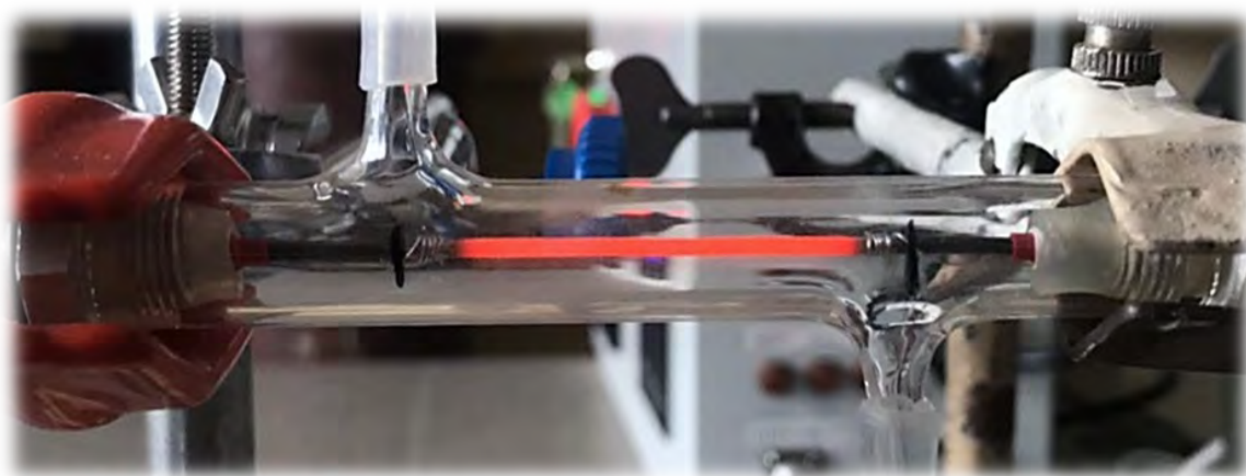
Figure 1. Microtubular membrane reactor for hydrocarbons conversion
