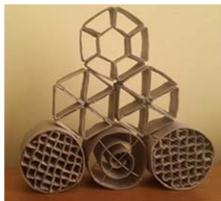
Fig. 1. Structured cartridges with fiber-glass catalyst, reinforced with metal gauze
