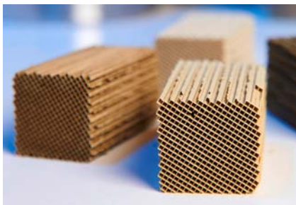
Figure 2: Ceramic monolith co-precipitated with NiAlZn catalyst.
