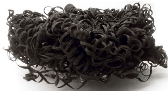
Figure 2. Carbon washcoated steel impregnated with ruthenium are used as structured catalyst materials for sugar hydrogenation
