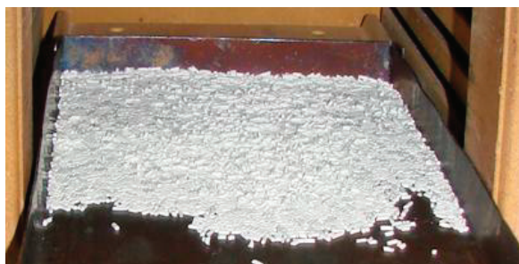
Fig. 1. Shaped SBA-15 cylinders after calcination.
