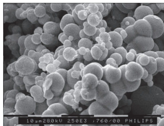
Figure 2. SEM image of tantalum carbide microspheres.
