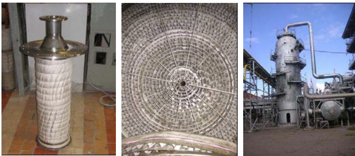
Figure 2: The device with radial bed of fiber-glass catalyst fabric for incineration of chlorinated VOCs (left), spiral-type catalyst block for purification of diesel exhausts (middle) and industrial reactor for incineration of VOC in waste gases (right)
