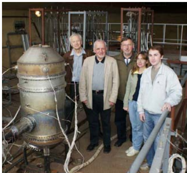
Fig.3. Scheme and photo of the prototype gas turbine catalytic combustor
