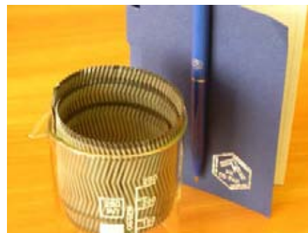
Fig. 3. The photos of the Pd-containing catalyst (50 mm x 500 mm) supported on corrugated metal foil.
