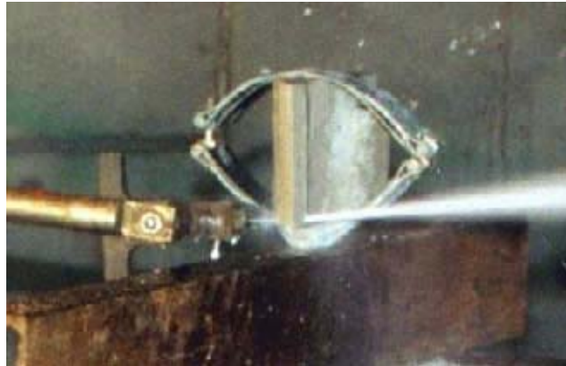
Fig. 2. SRP charge fragmentation by high-pressure toluene jets
