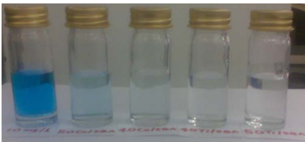
Figure 2. Degraded methylene blue solution under visible light using different catalysts.
