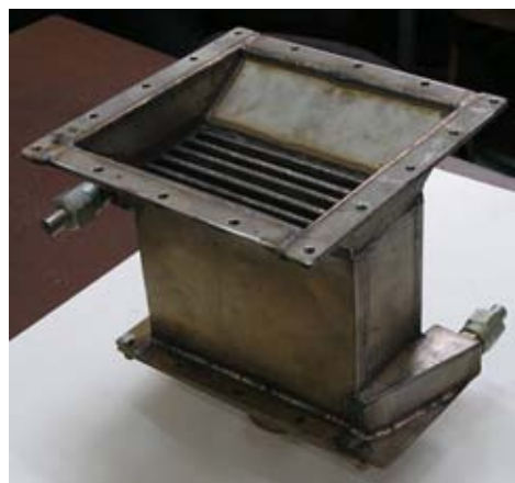
Figure 2: Milli-channel reactor with structured 10 wt.% Ni/CeO 2 catalyst for preferential CO methanation.
