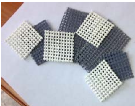
Figure 1. The glass fiber supports with pure and platinized TiO 2 Degussa P25.
