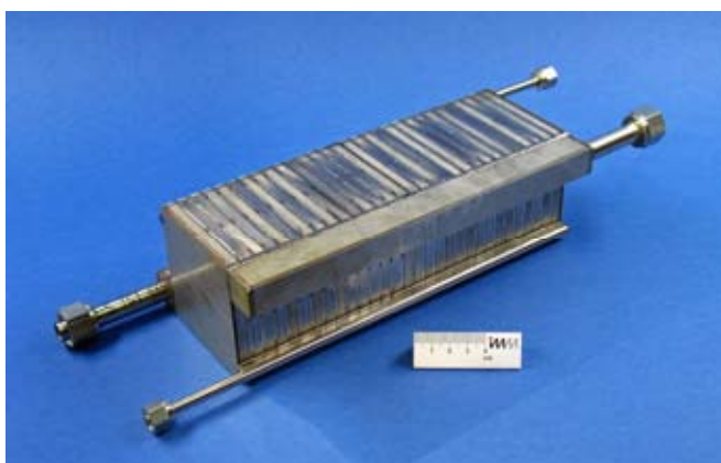
Fig. 1 Hot gas driven de-hydrogenation reactor
