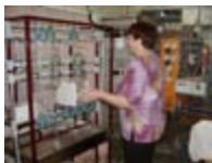
"CIRCULATION IMPREGNATION OF REFORMING CATALYSTS"
