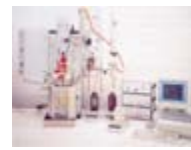
"CATALYSTS IMPREGNATION WITH AUTOMATIC SOLUTIONS PROPORTIONING"
