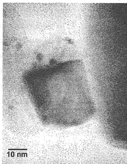
Fig. 3. TEM pictures of Pd/SiN-annl catalyst after reaction
