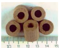
Thermostable catalyst ICT-12-40 for gas purification
