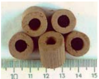
Thermostable catalyst ICT-12-40 for gas purification
