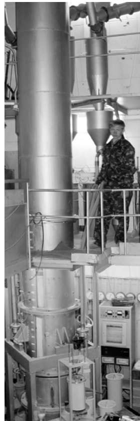
Cold flow model of 0.7 m ID
