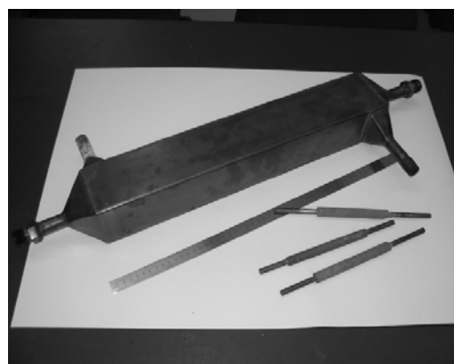
Reactor for hydrogen purification from CO
