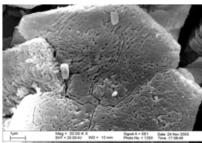
Dimensions and morphology of zeolite synthesized by traditional method (without support)
