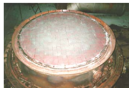
Reactor for ammonia oxidation with IC-42-1 catalyst (AO "Azot", Berezniki)
